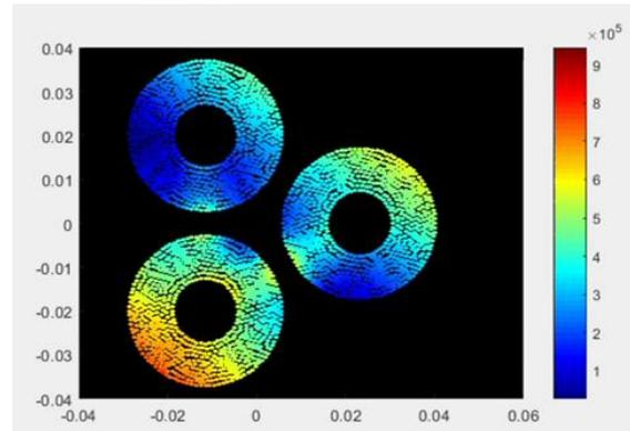
Figure 1: Von Mises Stress Distributions across Cable Insulation Layers at user defined point
