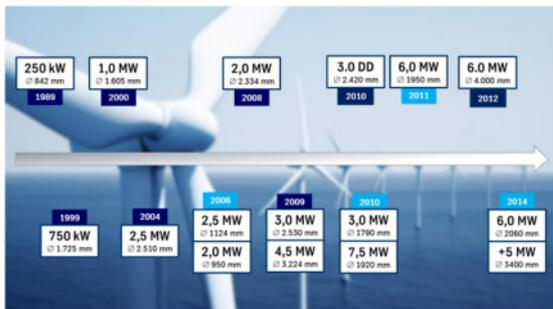
Fig. 1: tk Rothe Erde main bearing track record (<2015)
