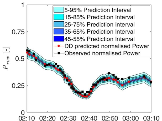
Fig. 1: Probabilistic forecast of wind power using remote sensing observations from a Dual-Doppler radar [2]
