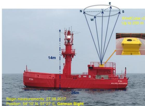
Fig. 1: Wind lidar mounted on the roof of the Lightship deckplatform.
