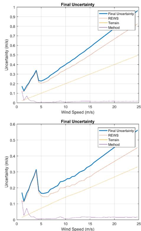
Fig 1: Final wind speed uncertainties and components for onshore case using LIDAR data only: applying the standard's methodology (top), and applying a revised methodology (bottom).
