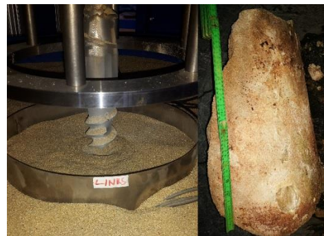
Fig. 2: Model tests with mechanical full displacement pile and excavated body after chemical injection
