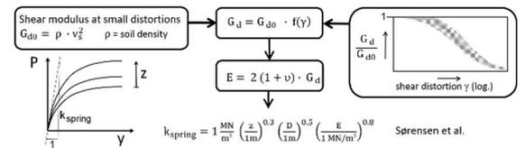
Fig. 2: Basic flowchart of pile-soil stiffness approach
