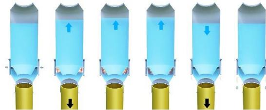
Fig. 2: Operating principle of the BLUE Hammer; from left to right: 1; Gas is fed into the combustion chamber, 2; Gas combustion creates a first blow and the water flows out of the combustion chamber, 3; Combustion continues and water column moves up, 4 Water column continues to move upward, 5; Water column falls back and delivers a second blow, 6; Exhaust gas is released through the exhaust valve.
