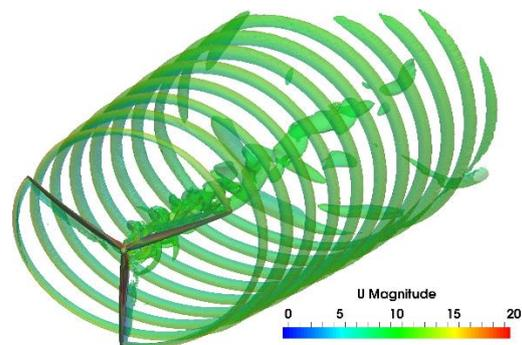
Fig. 1: Rotor wake structure
