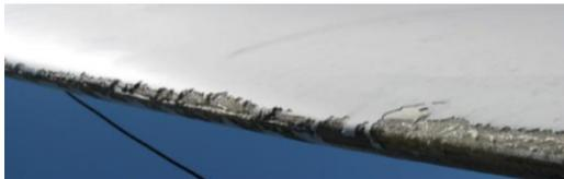
Fig. 1: An example of leading edge erosion [1]
