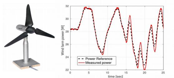
Fig. 2: A model wind turbine (left) and model wind farm following the power reference in wind tunnel experiments (right).
