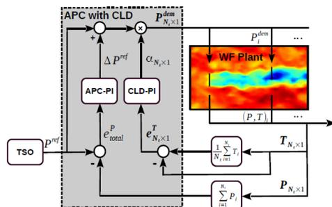
Fig. 1: Schematic illustration of the proposed APC of wind farms with coordinated load distribution (CLD).
