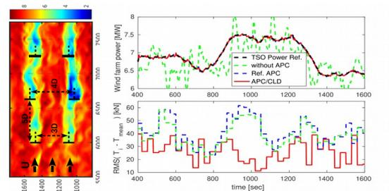
Fig. 3: A 2x3 wind farm layout in LES (left) and total power and root mean square of errors between 30-sec averaged applied thrusts and their mean value (right).
