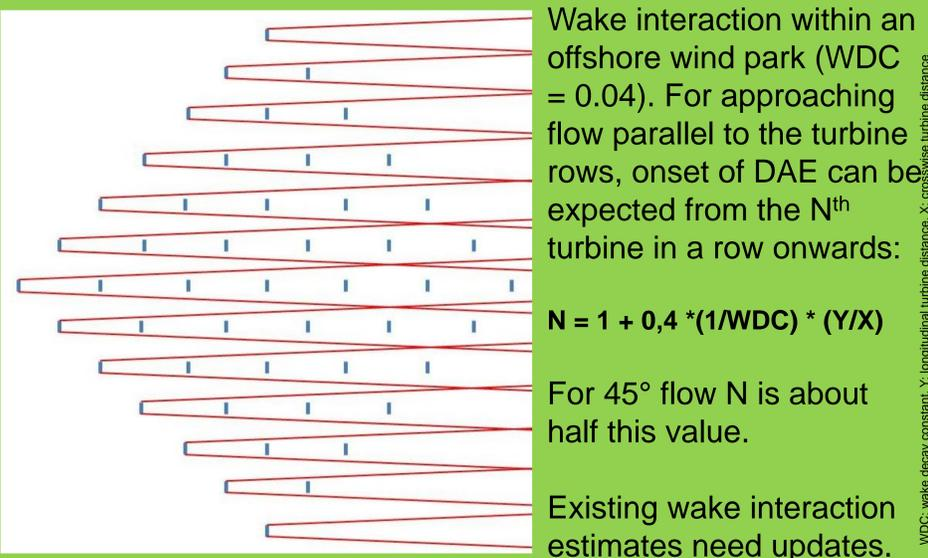
**Offshore wind park wakes:** The wind park parameterization in WRF [2] has been evaluated [3] in WIPAFF [4]. It is working well and the exact choice of parameters within the parameterization is less important than the correct simulation of the undisturbed upwind wind conditions. This becomes especially important for wind parks close to shore lines.
