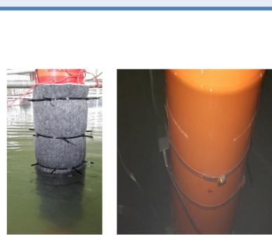
Fig. 3: Application of Marine Growth (Left) and Damage (Right)
