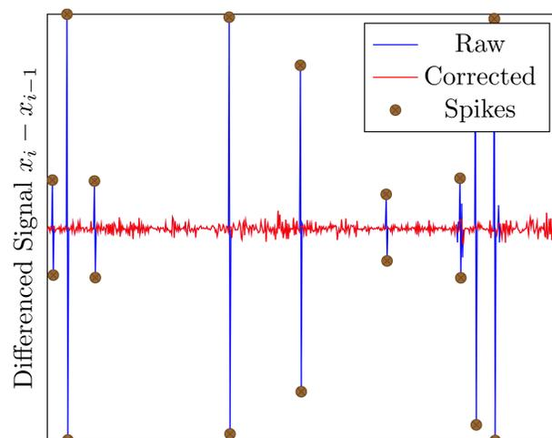
Figure 3: The differenced ( $x_n - x_{n-1}$ ) signal shown in Fig. 2 compared with the corrected (despiked) signal and the identified spikes with consecutive minimum/maximum values.
