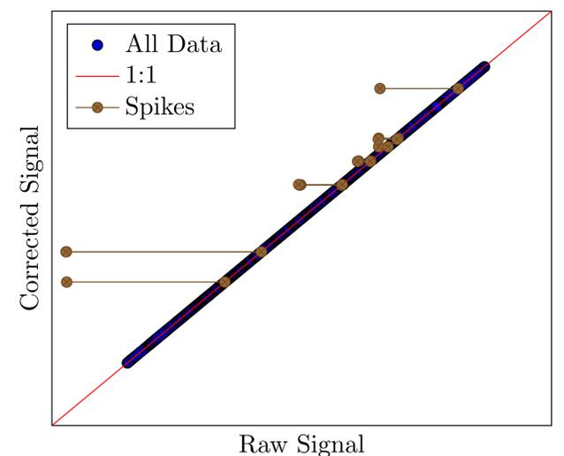
Figure 6: Correlation between the raw and corrected signals shown in Fig. 4, with the spikes indicated relative to the 1:1 line ( $r = 1$ ), where the correlation coefficient  $r$  defined by Eq. 1 is used to evaluate the quality of the raw signal. Here,  $r = 0.74$ .
