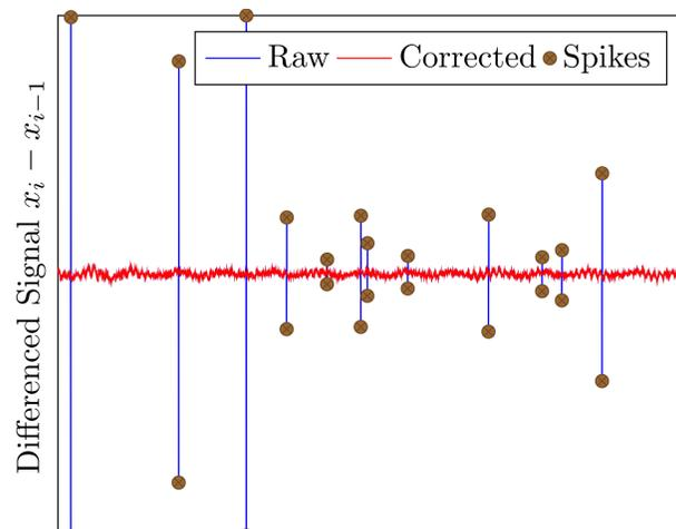
Figure 5: The differenced ( $x_n - x_{n-1}$ ) signal shown in Fig. 4 compared with the corrected (despiked) signal and the identified isolated spikes.
