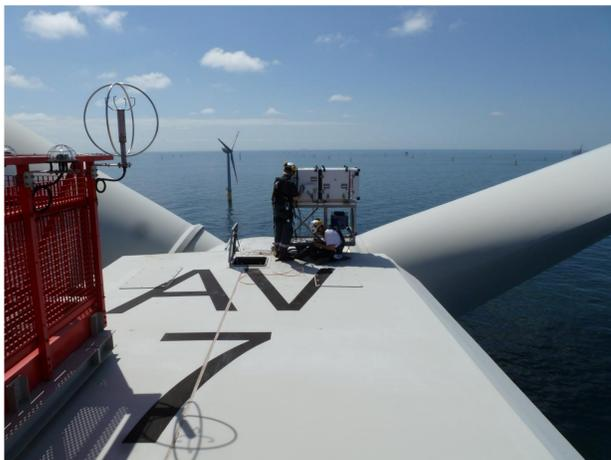
Figure 1: Long-term offshore-measurement campaigns involve a wide range of sensors tracking the meteorological, oceanographic and structural effects within wind farms.
