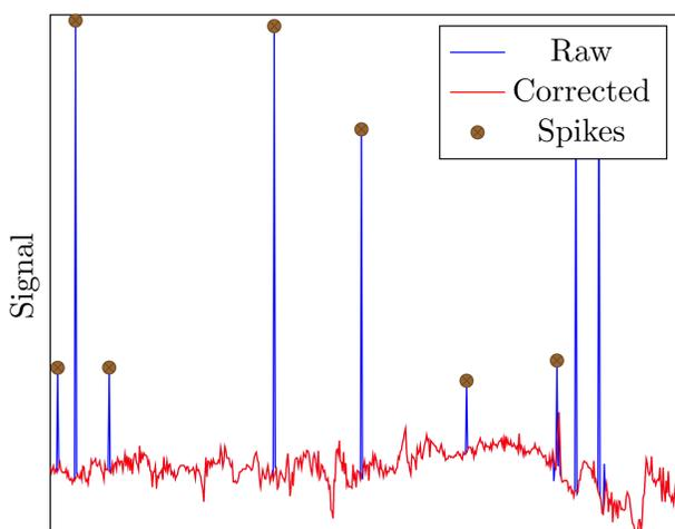
Figure 2: Signal containing spikes in comparison with the corrected signal. Outlier or spike events are indicated by points.
