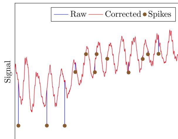
Figure 4: Signal containing spikes embedded within the sinusoidal behaviour compared with the corrected signal. Plausible spike events are indicated.
