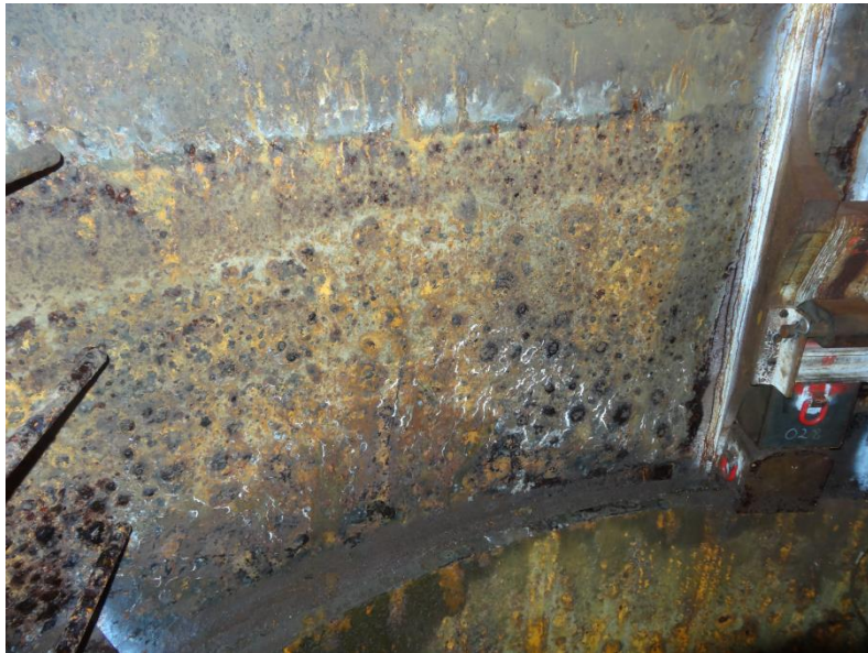
Insufficient inner corrosion protection
