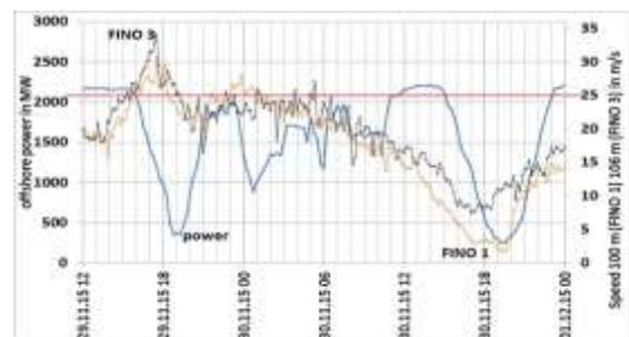
Fig. 3: North Sea offshore power output (bold blue line), 100 m wind speed at FINO 1 (thin orange line) and 106 m wind speed at FINO 3 (thin black line) for 29-30 Nov 2015.
