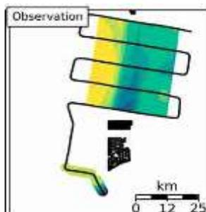
Fig. 2: Measured wind speed at hub height (90 m) behind a wind park cluster in the North Sea. Yellow: 9 m/s, blue: 6 m/s. From [2].
